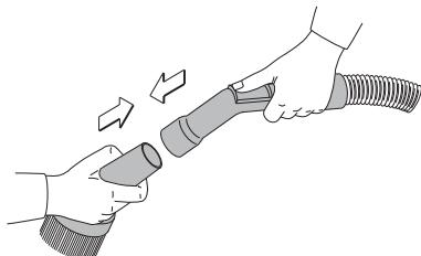
Fit the appropriate cleaning accessory on the flexible hose.
