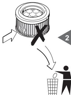
Check if the surface of the cartridge is torn; in this case, the filter cartridge cannot be used any longer.
